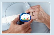
Twist the end of the cannula clockwise onto the Cannula connector on SleepView® until snug.
